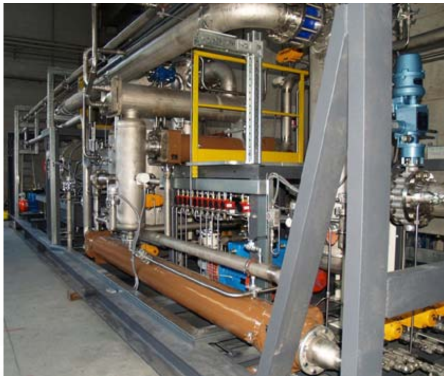
GAS-COOLER, GAS-HEATER and OIL-COOLER in gas compressor station
