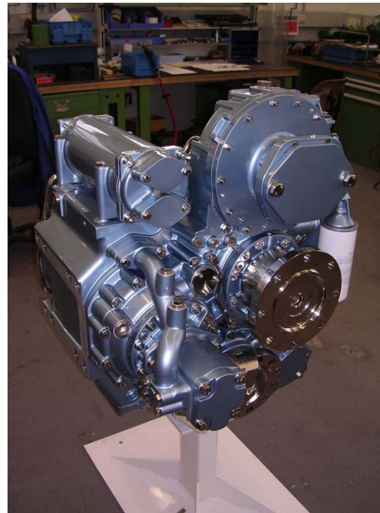
Standard OIL-COOLER directly mounted on marine gear box
